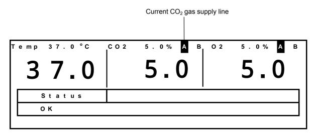
**5.** The MCO-21GC detects that there is no more  $CO_2$  gas in a cylinder when the  $CO_2$  density in the chamber does not increase for a while even after opening the  $CO_2$  gas valve in the Incubator. It switches the gas supply line when it detects that there is no more gas. At that time, the following indications of switching the gas cylinder are provided.
